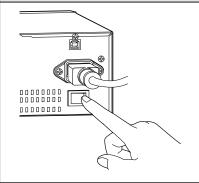
Press the **POWER** switch on the rear panel to turn on the power.
