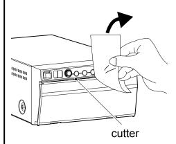
Cut the paper end with the cutter by pulling the paper upwards against the cutter blade. ■ When setting the paper, observe the following precautions to prevent paper jam.
