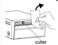
Cut the printed paper with the cutter by tearing off the paper in the upper right direction.
